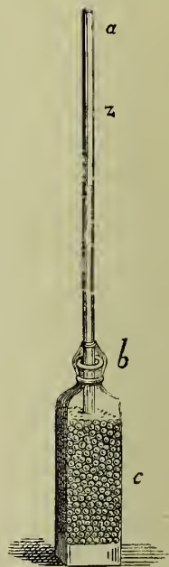
Fig. 23.—Measurement of the elastic force of the gas produced by fermenting peas.
